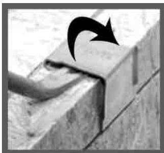
The clip can be taken off easy with a screwdriver. Just put it into the bending ups of the clip and **with a rotation** the clip is levered from the groove.
