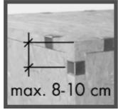
Insert into the groove on one side of the box, press across the corner and hit with a hammer (min.300 g) (slight clicking noise = perfect fit!)
